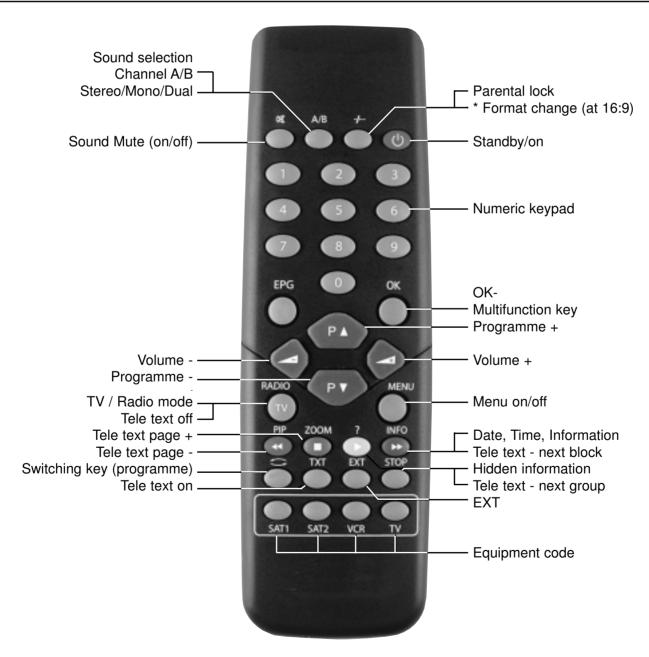
Important! Press the **TV** key at bottom right after each time you have changed the batteries!
